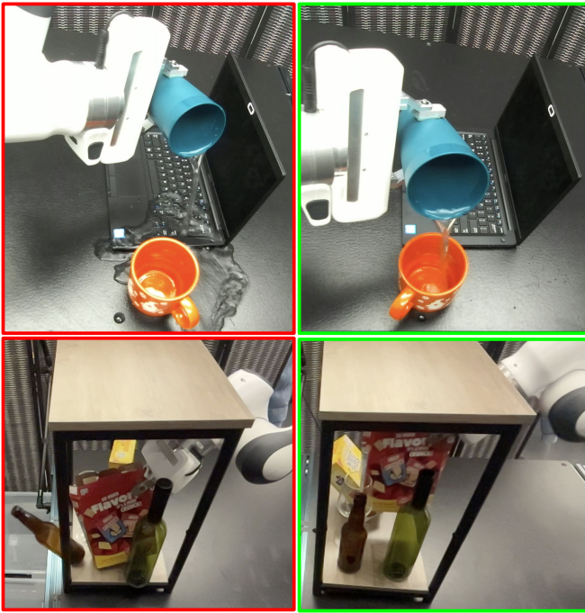
Fig. 9: Sim-to-real transfer of policies trained in OOPSIEVERSE. We evaluate baseline IL policy (without health feedback) with the IL policy with health-filtered episodes on Panda robot. The baseline IL policy often performs unsafe behaviors like spilling water on the laptop or pushing a fragile bottle over the shelf. Whereas the damage-aware filtered-episode IL policy learns safer behaviors. The damage-aware IL policy results in a 60 % safer execution as compared to the baseline IL policy. This shows that OOPSIEVERSE can enable transferring safer policies to the real world.
