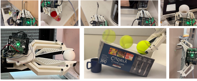
Fig. 5: Experimental evaluation for task versatility. BaRiFlex is mounted on a portable device and used by a human to perform multiple household tasks including a full long horizon activity, prepare a cup of instant coffee that involves tasks such as (top row, left-to-right): opening cabinets, opening jars, pinch-grasping utensils, pressing buttons, grasping delicate plastic cups. We also evaluated other tasks such as grasping an egg, catching a fast-moving object, and opening heavy doors (Bottom row). Through this human-controlled manipulation, we empirically evidence the high task-variability enabled by BaRiFlex, which covers a significant fraction of possible tasks in household domains.
